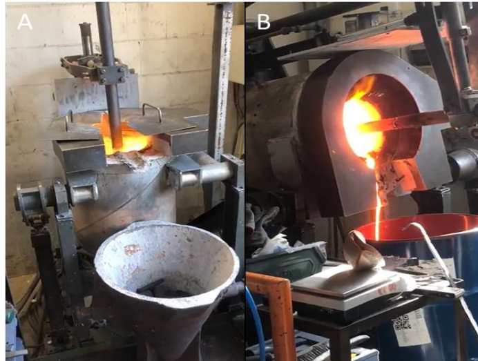
Figure 1A. Smelting of the BR mix with the EAF and Figure 1B. Quenching of the slag in water.
